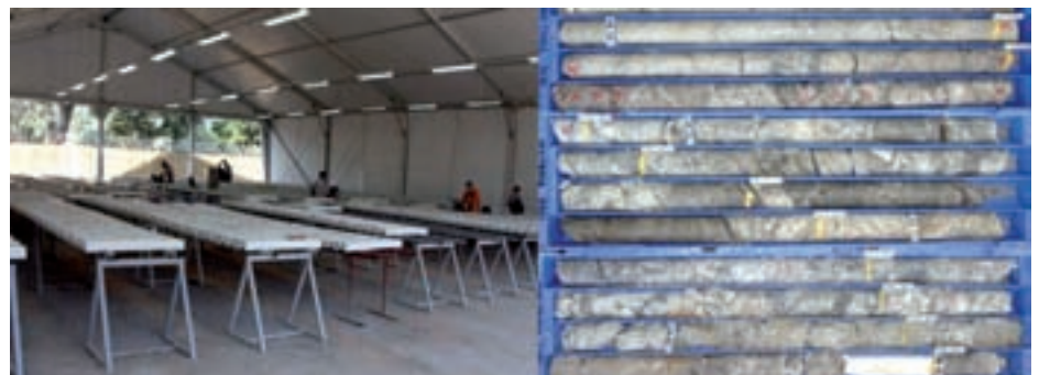
Core-logging facility at WMZ's headquarters near Bejaia and high-grade mineralised core from Tala Hamza
